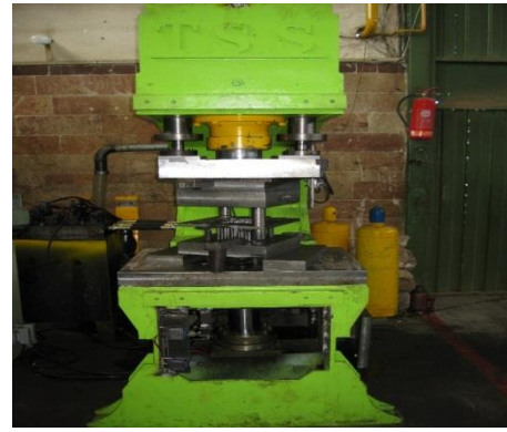
Fig. 1: Dual-purpose hydraulic press T.S.S and assembled multi-point die.
